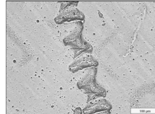
Figure 15. Residual trail mark on emulsion.
