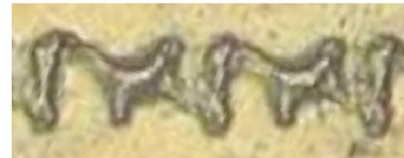
Figure 15. Residual trail mark on emulsion.
